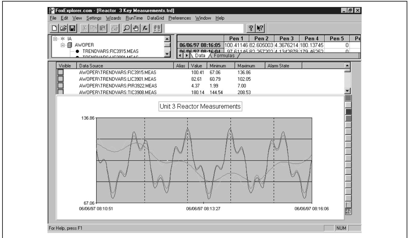
AIM\*Explorer is a PC desktop tool for visualizing and exploring real-time and historical process data served from I/A Series systems and other data servers. AIM\*Explorer features three different window types: Real-time trends (above) that dynamically track up to 16 data objects; charts of historical data from multiple historians; and Batch™ events that compare completed batches monitored by AIM\*Track™ and the I/A Series Batch Set.
