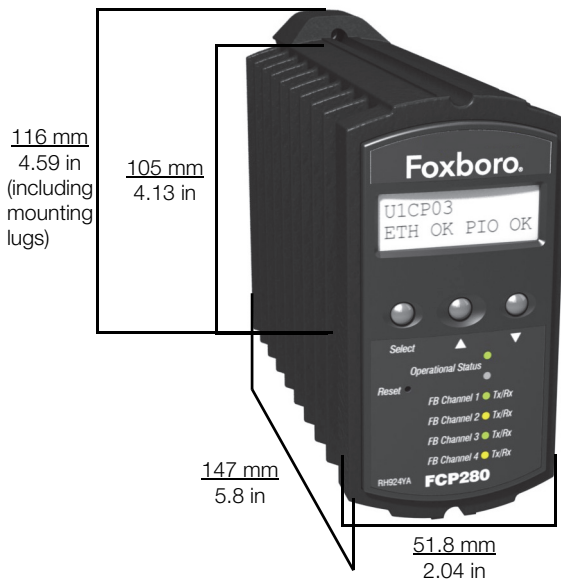
Figure 6. FCP280 Dimensions
