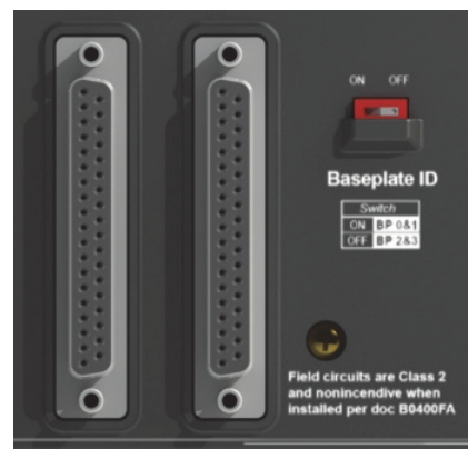
Figure 2. Compact 200 Series Baseplate ID DIP Switch
