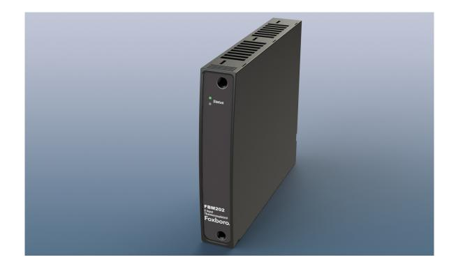
The Compact FBM202 Thermocouple/mV Input Interface contains eight thermocouple input channels, and one isolated RTD reference junction compensation channel.
