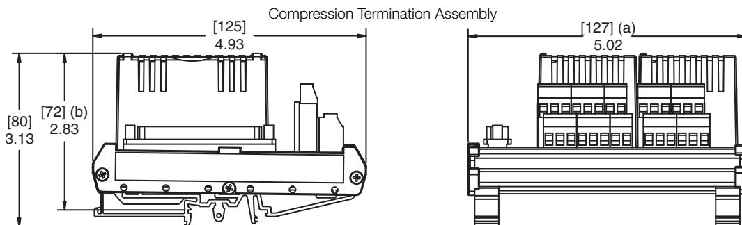
(a) Overall width – for determining DIN rail loading.
