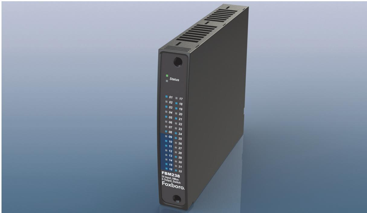
Many plant situations, such as Motor Control Center controls, require several inputs for each output. The Compact FBM238 contains 24 discrete input and eight discrete output channels that are compatible with voltages and currents commonly found in industrial plants. An external power supply is used to energize the field circuits.
