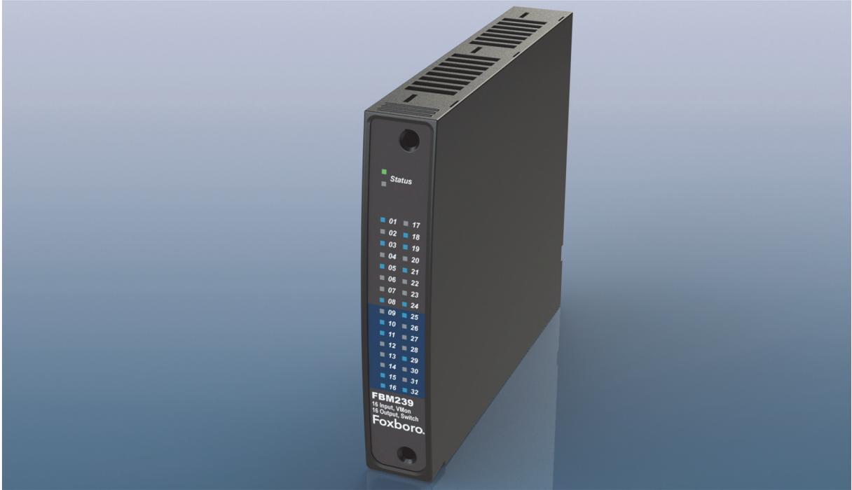
*The Compact FBM239 contains 16 discrete input and 16 discrete output channels that are compatible with voltages and currents commonly found in industrial plants. An external power supply is used to energize the field circuits.*
