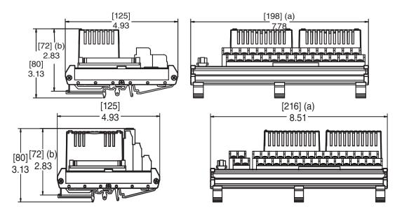
(a) Overall width – for determining DIN rail loading.
