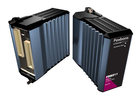
The FBM211, 0 to 20 mA Input Module contains sixteen 20 mA DC analog input channels.
