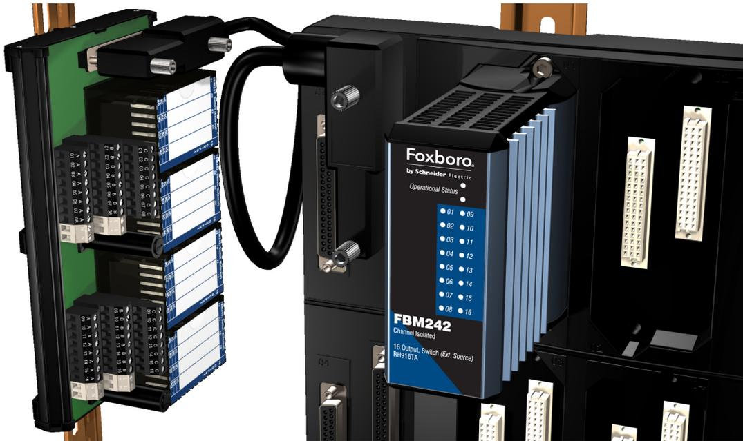
*The FBM242 contains 16 discrete output channels that are compatible with voltages and currents commonly found in industrial plants. An external power supply is used to energize the field circuits.*
