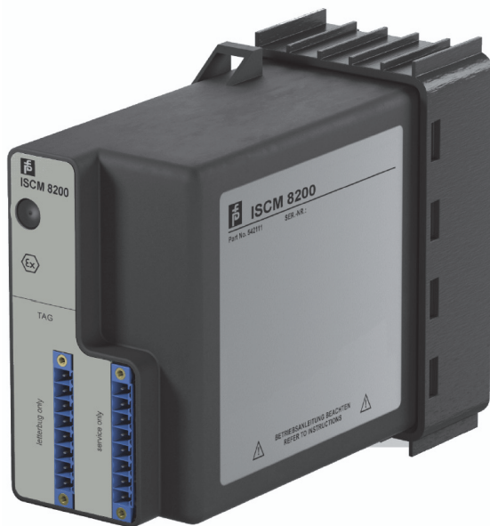
Figure 7. Intrinsically Safe Communication Module for Zone 1 (FB-Style) Applications (P0927BW/P0924GU)
