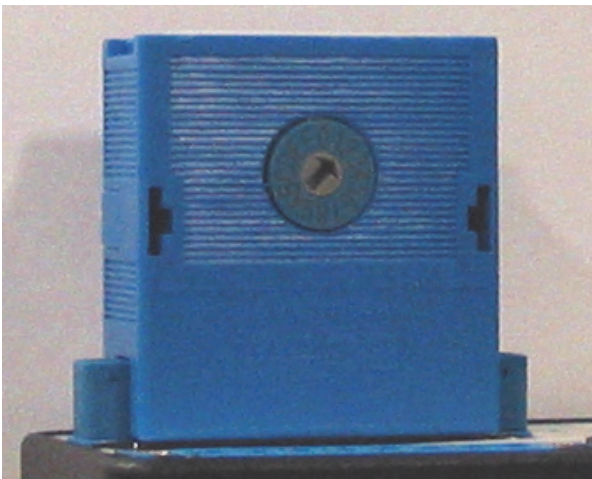
Figure 8. Station or Module Name Rotary Switch Module (P0924GV)
