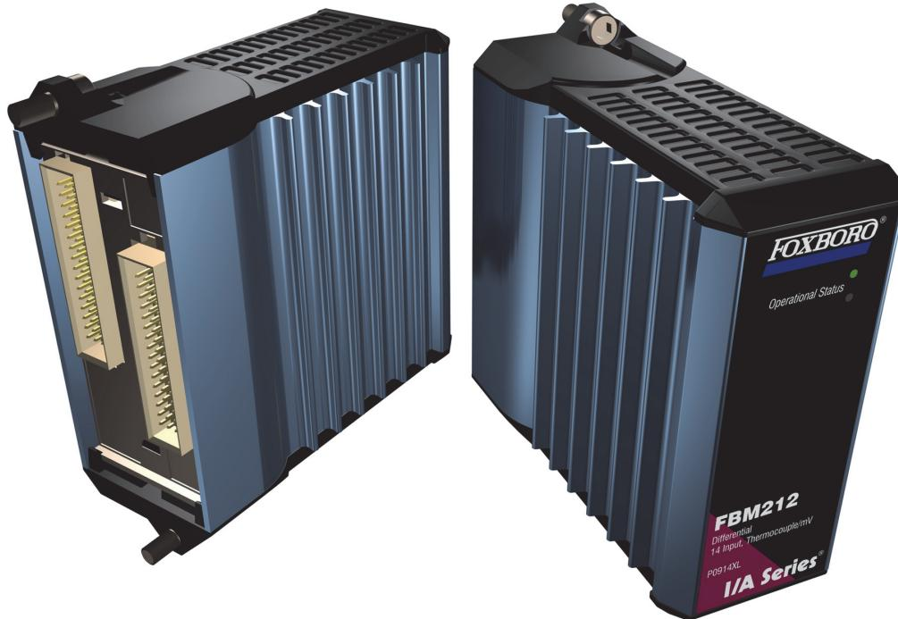
The FBM212 Thermocouple/mV Differential Input Module contains 14 differentially isolated thermocouple input channels, and one differentially isolated RTD reference junction temperature compensation channel.
