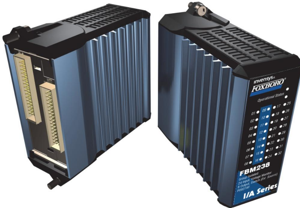
Many plant situations, such as Motor Control Center controls, require several inputs for each output. The FBM238 contains 24 discrete input and eight discrete output channels that are compatible with voltages and currents commonly found in industrial plants. An external power supply is used to energize the field circuits.
