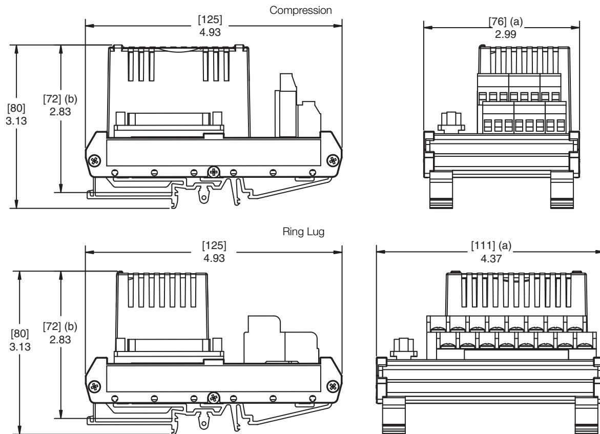
(a) Overall width – for determining DIN rail loading.
