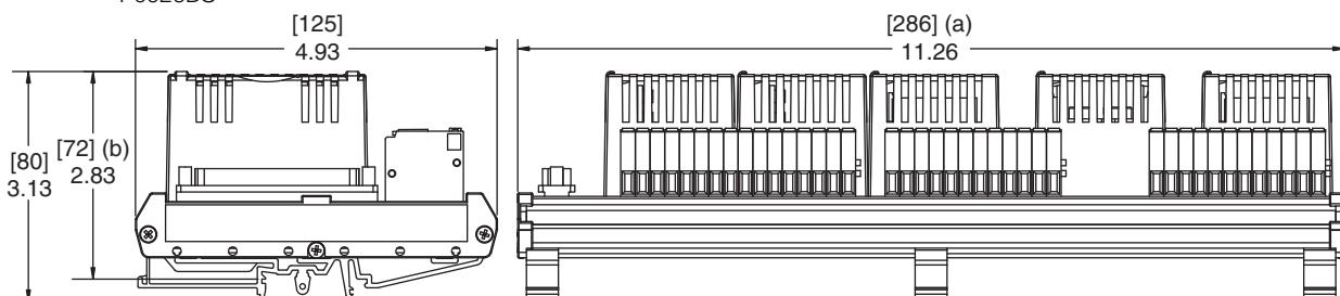
(a) Overall width – for determining DIN rail loading.
