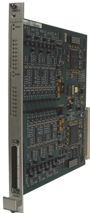
*Foxboro Evo™ distributed control system (DCS) Fieldbus Modules (FBMs) allow migration from Fisher PROVOX® process input and output (I/O) components to a Foxboro Evo process control system.*
