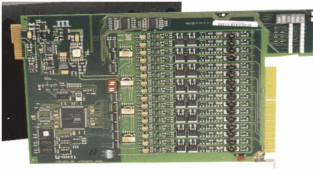
The Foxboro Evo™ Control Processors and distributed control system (DCS) Fieldbus Modules (FBMs) replace the Westinghouse WDPF® I or II Controllers and Q-Cards, respectively, and connect existing field devices to the Foxboro Evo system.
