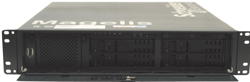
Critical software processes are often placed onto stand-alone workstations, with redundancy provided through replicating that configuration. This permits continued plant operation during maintenance as well as in the unusual event of a workstation failure. The compact format of the Magelis M92 workstation permits much better use of plant physical volume. Its industrial design supports 24/7 operation at 40 DegC.
