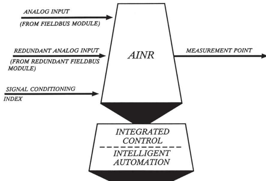
*Redundant Analog Input (AINR) block scans and filters redundant analog inputs coming from a pair of redundant Fieldbus Modules supporting either a single transmitter or dual (redundant) transmitters for selection of a single field measurement.*
