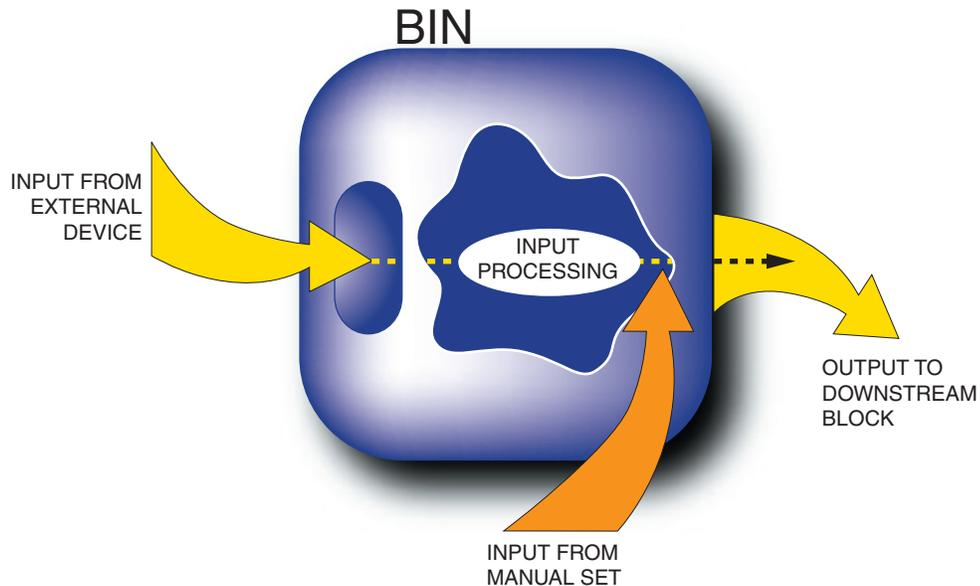
*The Binary Input (BIN) block is a Distributed Control Interface (DCI) block. (DCI blocks support connectivity of I/A Series control stations to various bus resident devices via a general purpose interface.) The BIN block provides the control strategy with the capability to read a single binary value, having two states such as ON and OFF or START and STOP, from an address in an associated Fieldbus Module (FBM).*
