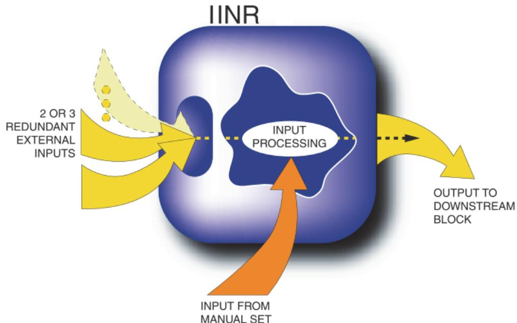
The Redundant Integer Input (IINR) block enables the control strategy to read a single integer value selected from multiple points in the same or different field devices.
