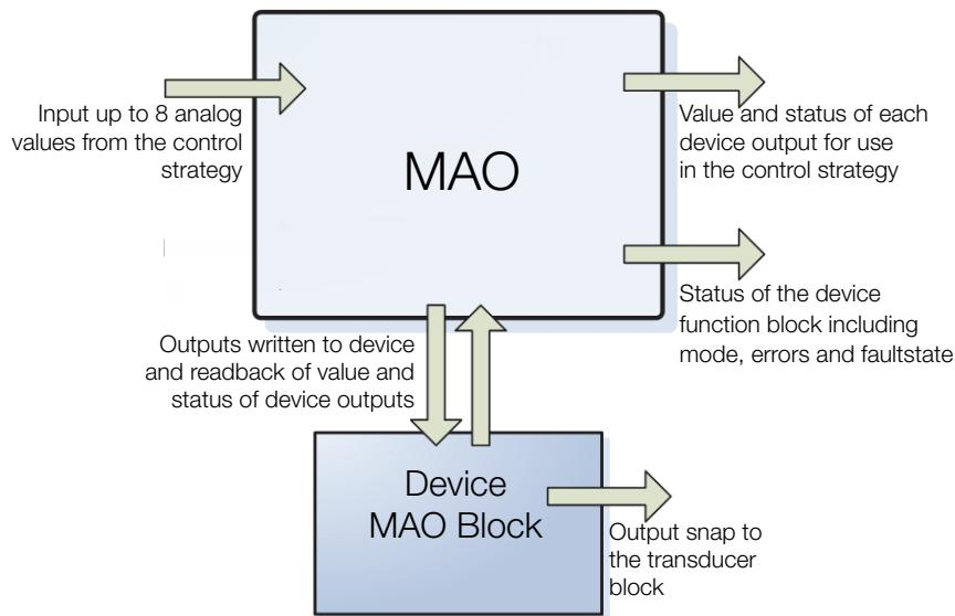
The Multiple Analog Output (MAO) block enables the control strategy to write up to eight analog values to an MAO device function block operating in a FOUNDATION fieldbus™ H1 device.
