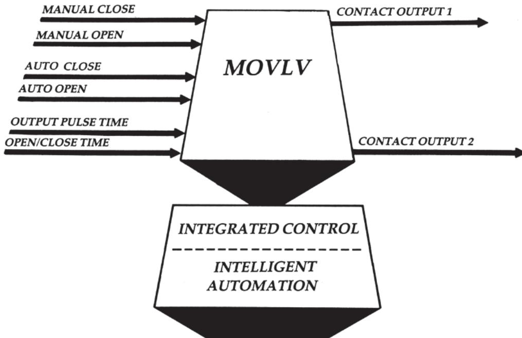
The MOV LV block provides control of a 3-wire motor operated control valve. The 3-wire configuration provides two pulsed outputs.
