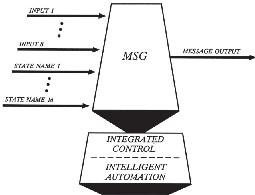
Message Generator (MSG) block generates state change messages for Intelligent Field Devices and control schemes requiring simple message generation.
