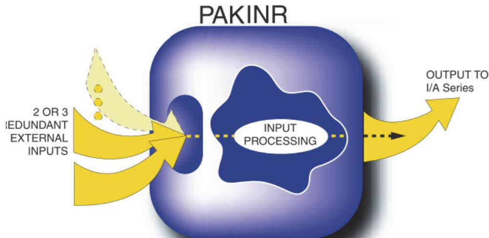
*The Packed Input (PAKIN) block reads up to 32 bits of discrete data from a group address selected from multiple points in the same or different field devices.*
