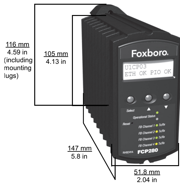
Figure 10 - FCP280 Dimensions
