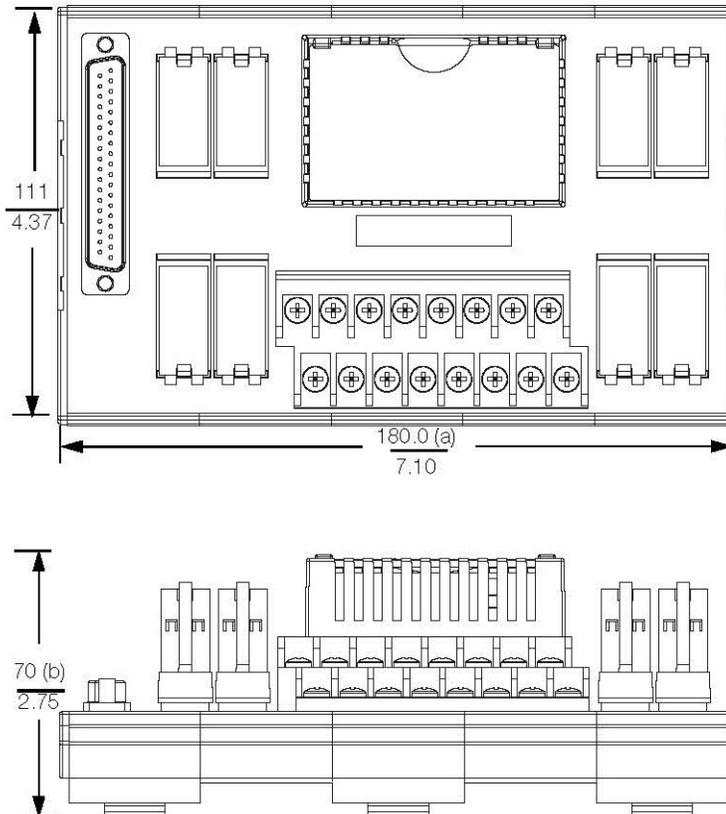
(a) Overall width – for determining DIN rail loading.
