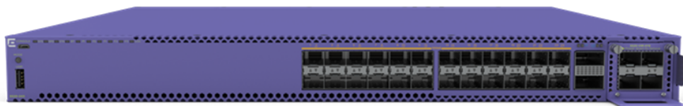
Figure 1 - 24-Gigabit (SFP+) 5520 Managed Switch (RH102BF)
