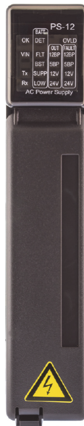
Figure 5 - SCD2200 Power Supply Module
