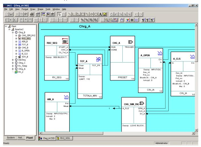
Physical I/O is associated with the CSD by dragging the equipment control block (ECB) object of the appropriate I/O module represented in the Navigator Pane onto the CSD drawing in the Editor Pane. Once the ECB object is dragged, the parameters from the referenced ECB can be connected to the appropriate parameters in the I/O function blocks on the CSD.
